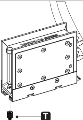
\*If M.2 SSD is already installed on the motherboard with a copper pillar, using **T** will not be necessary.
